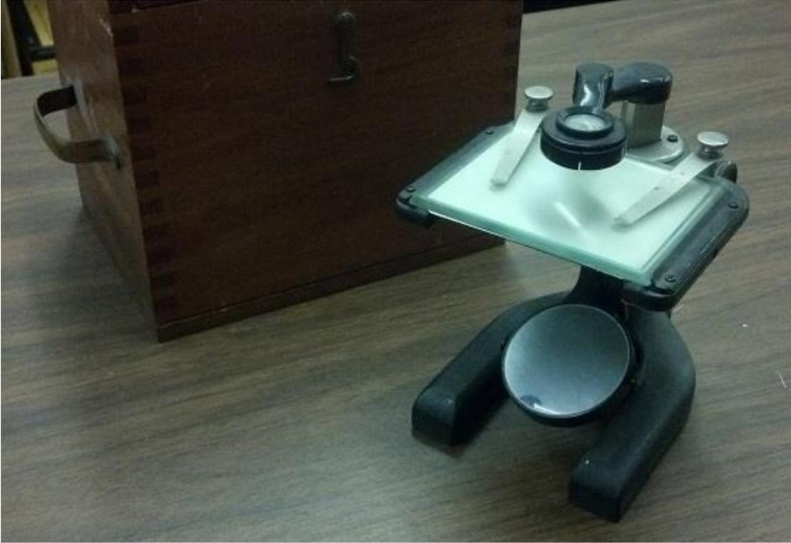
This microscope was used to view three dimensional objects and was chiefly designed for botanical dissecting but could also be used for general dissecting purposes. The design is based on the American Microscope maker Joseph Zentmayer's botanical dissecting microscope design. It was most likely used at the College for student instruction.
